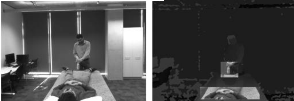
Figure 5. Left: video (RGB) image of the actual scene. Right: processed depth imagery of the same scene.
